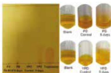
Figure 1. Qualitative analysis for the detection of alkaloids in extracts of Phanerodontia sp. BRM 62389. On the left, chromatographic profile obtained by Thin Layer Chromatography (TLC) using Dragendorff's reagent for visualization.
