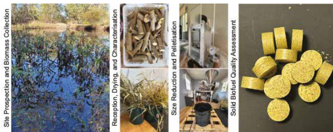
Figure: Schematic of the pathway for converting weed biomass into solid biofuel.
